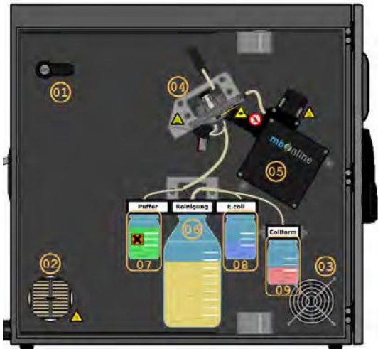
Figure 6: The internal operation side of the mB-Online Coliguard® analyzer
